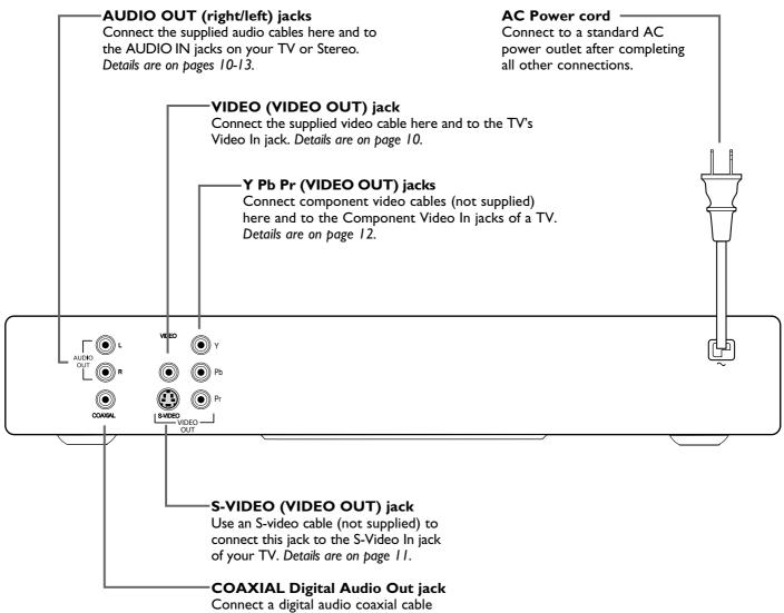
Connect a digital audio coaxial cable (not supplied) here and to the Digital Audio Coaxial In jack of a Stereo. Details are on page 14.
